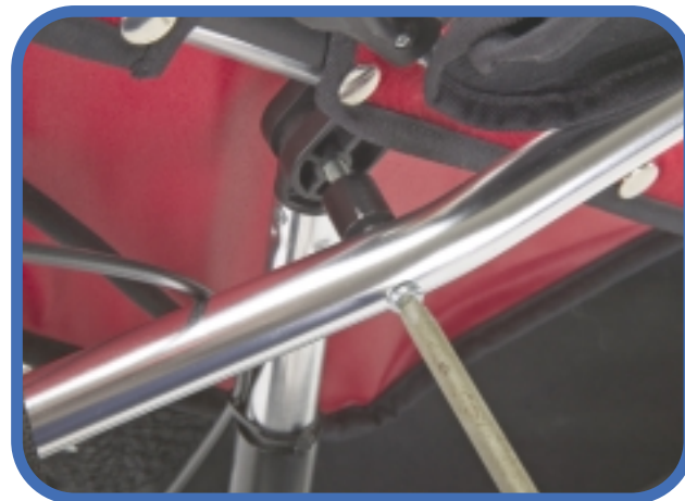
3. Locate upright on Jogger. Remove existing bolt from upright using philip head screwdriver, align car seat adapter hole with upright on jogger and secure with hardware supplied.
